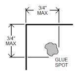
g. Continuous glue lines may be used as cover-to-cover seals and must be placed along the entire length of the open edge and end no more than 3/4-inch from the open ends (see Exhibit 201.3.11.g).
